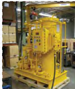
Ex: Portable, Carbon steel heated system with 2 Pre-filters. Explosion-Proof; rated for Group B (Hydrogen) atmosphere. 2008
